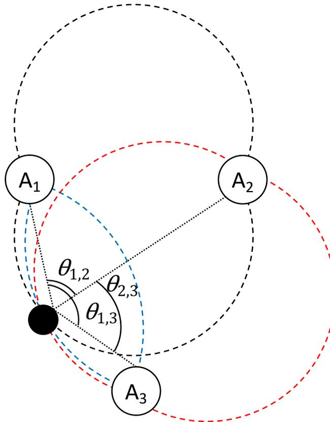
Angle difference between 3 pairs of anchors.
