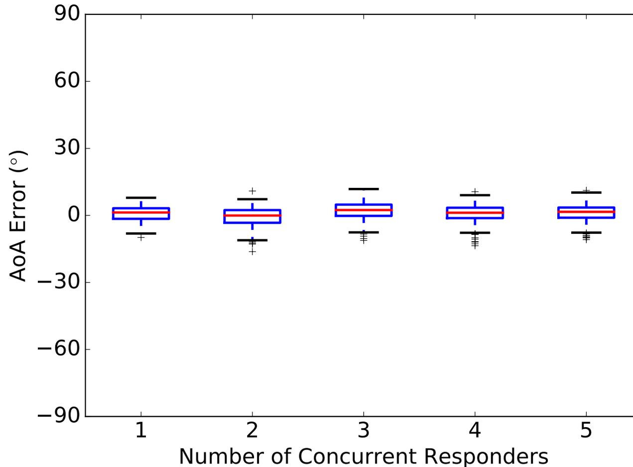
Concurrency does not significantly affect AoA estimation when adding more anchors showing 100 measurements per box plot. Number of receiver tags are still unlimited.
