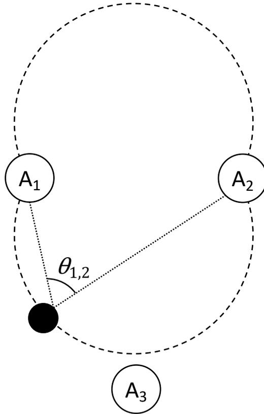
Angle difference between 1 pair of anchors.
