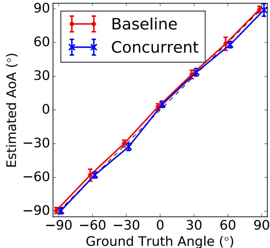
Concurrency does not significantly affect AoA estimation in different angles (100 measurements per data point)
