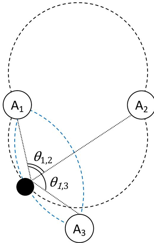
Angle difference between 2 pairs of anchors.
