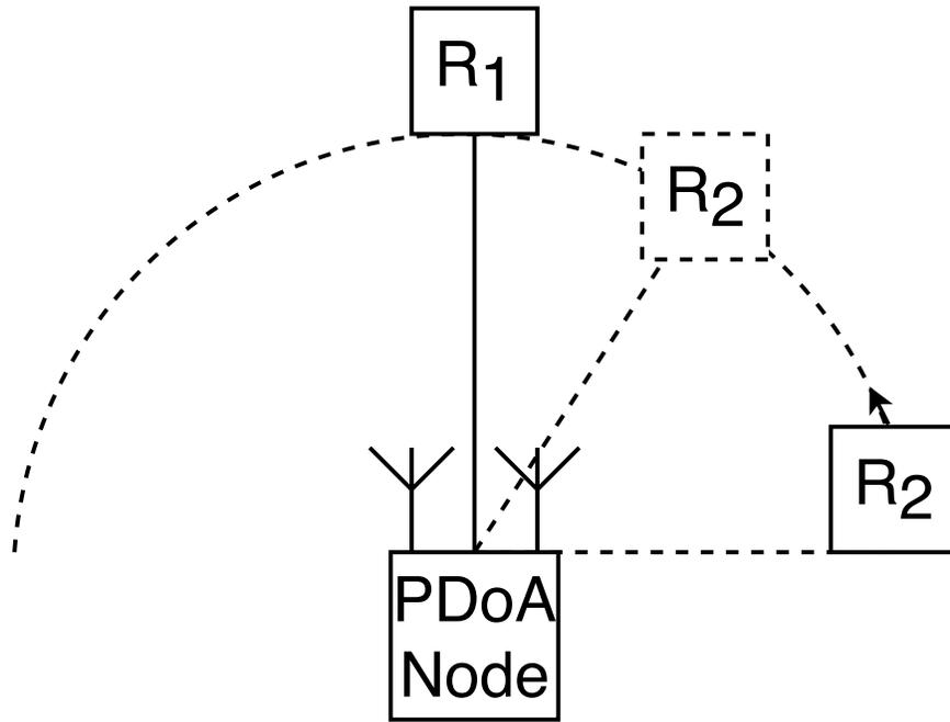
We change angle of one responder when the other one is static. Dipole antenna performance expected to degrade near extreme angles.
