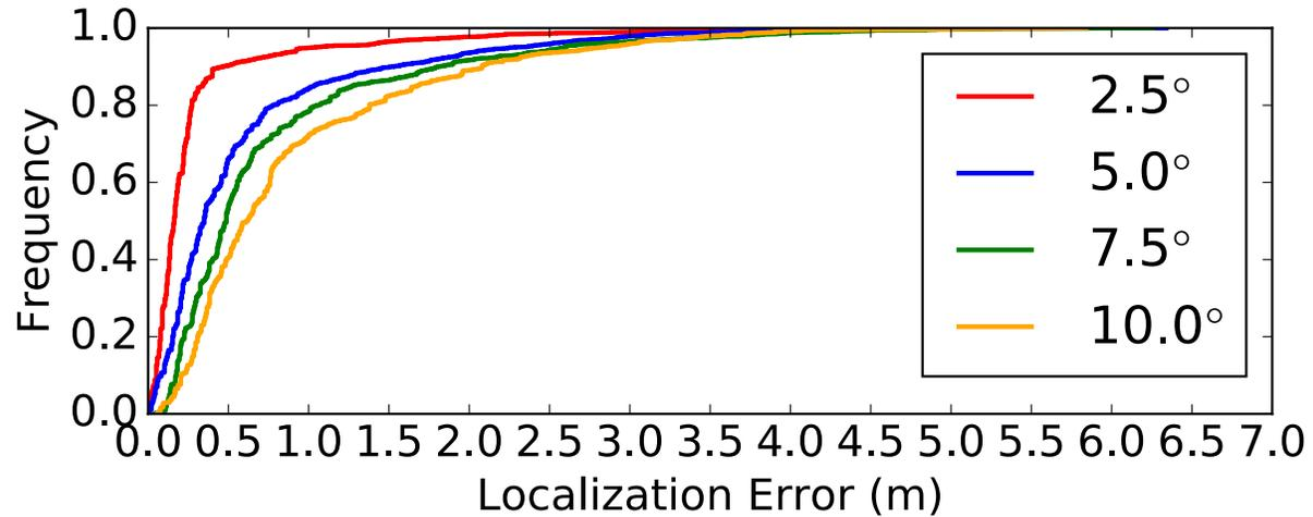
CDF of localization error, simulated for different noise levels.
